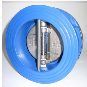
Dual Plate Wafer Check Face-to-face: EN558 Series 16 Size: DN40-DN800 Max W.P.: 16bar Ends Drilling: PN10, PN16, ANSI150
