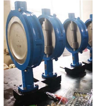
Connection: Wafer or Lug Double Eccentric, PTFE Seat Size: DN50-DN600 Ends Drilling: PN10, PN16, PN25, PN40, CL150-CL300
