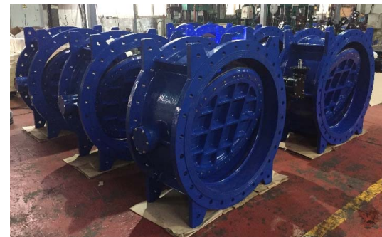
Connection: Double Flanged Double Eccentric, rubber seat Face-to-face: EN558 Series 14 Size: DN100-DN2000 Max W.P.: 25bar Ends Drilling: PN10, PN16, PN25, ANSI150
