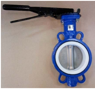
Connection: Wafer or Lug One-Piece Body, PTFE seat Face-to-face: EN558 Series 20 Size: DN40-DN600 Max W.P.: 10bar Ends Drilling: PN10, PN16, ANSI150
