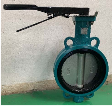
Connection: Wafer Face-to-face: EN558 Series 20 Size: DN25-DN1000 Max W.P.: 16bar Ends Drilling: PN10, PN16, ANSI150
