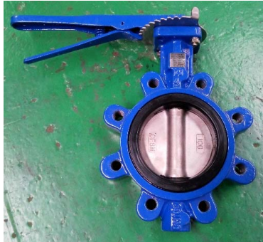
Connection: Lug Face-to-face: EN558 Series 20 Size: DN40-DN1000 Max W.P.: 16bar Ends Drilling: PN10, PN16, ANSI150
