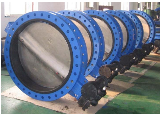
Connection: U Flanged Face-to-face: EN558 Series 20 Size: DN50-DN2000 Max W.P.: 16bar Ends Drilling: PN10, PN16, ANSI150
