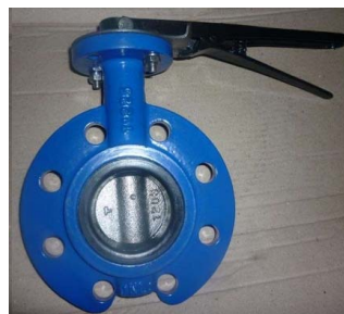
Connection: Wafer Face-to-face: EN558 Series 20 Size: DN50-DN600 Max W.P.: 25bar Ends Drilling: PN25
