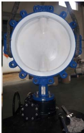
Connection: Wafer or Lug 2 pcs Split Body, thick PTFE seat Face-to-face: EN558 Series 20 Size: DN40-DN800 Max W.P.: 16bar Ends Drilling: PN10, PN16, ANSI150
