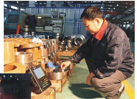
Ultrasonic Testing and Dye-penetrant Testing
