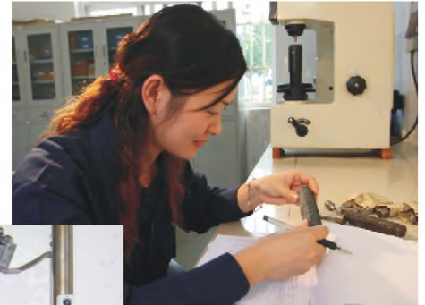
API591 Stem to Wedge Connection Testing (Physical Properties)
